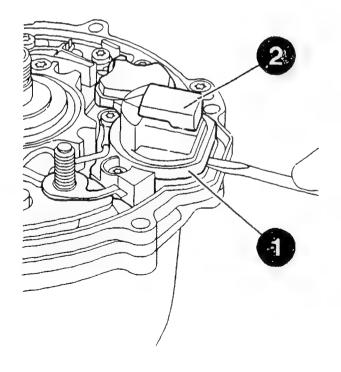
DISMANTLING AND CHECKING ALTERNATOR Dismantling regulator Unfasten DF connection (1). Unfasten connection/terminal V (2). Slacken off bolts (3) of regulator (4). TORX 720: comm. avail.
